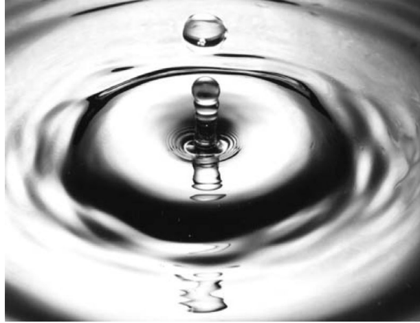
FIGURE 14. An oblique view of a falling water column for the initial conditions of d_D = 6.2 mm, Fr = 130 and We = 663 ( Bo = 5.2 ). Drop separation occurs and air bubbles are observable at the bottom of the drop. The column base is not deep but free surface swelling can be clearly seen.
